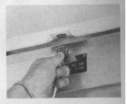
16 the slots in road cover and turn latch handles until bed roof is secure. Secure latches by folding the handles flat.
