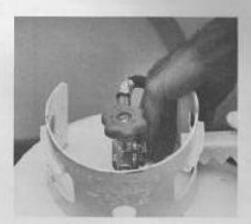
This is the knurled screw on the side of the main valve body. It is opened and closed by hand without pliers or wrenches. After you have your bottle filled, open the 10% valve. This should be done in an open area, away from any flame. You will hear a loud hissing from the gas escaping. If you see a white-frosty vapor coming out, the bottle is over-filled. Allow this to discharge until invisible and close the valve. The bottle is now properly filled. Keep hands away from vapor.
