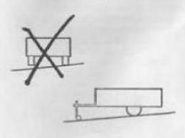
2 Detach safety chains, electrical hook-up, and slip tongue jack wheel over jack sleeve (locking pin on wheel fits into slot in sleeve).
