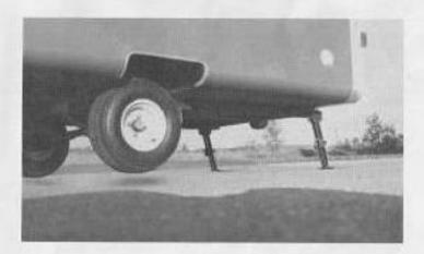
CAUTION: Raising the trailer on the leveling legs and tongue jack wheel, as described above, is intended for tire-changing purposes only. If it is necessary to work under the trailer, place additional supports under all four corners of the frame. Never use a bumper jack.
